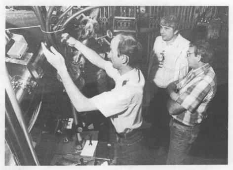
PREPARING EXPERIMENT — Russian scientists Georgyi Volkov (left) and Eugeni Grabovski (center) and Sandia experiment coordinator Johann Seamen (1273) work on a line-of-sight diagnostic tube underneath the Saturn accelerator.
